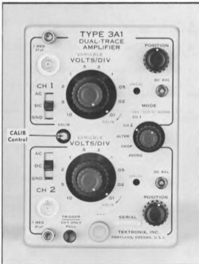
Fig. 7-11. Location of front panel CALIB control.
